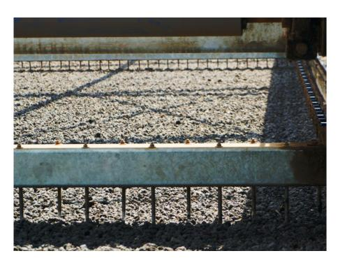
With options for automatic conveying and manual input, the Naturetech and i+M system offers flexibility right from the start. With the help of a thin sludge layer in combination with fast turning intervals and optimum air supply the Naturetech and i+M technology prevents anaerobic layers and charges fresh air with evaporated water in a continuous process.
